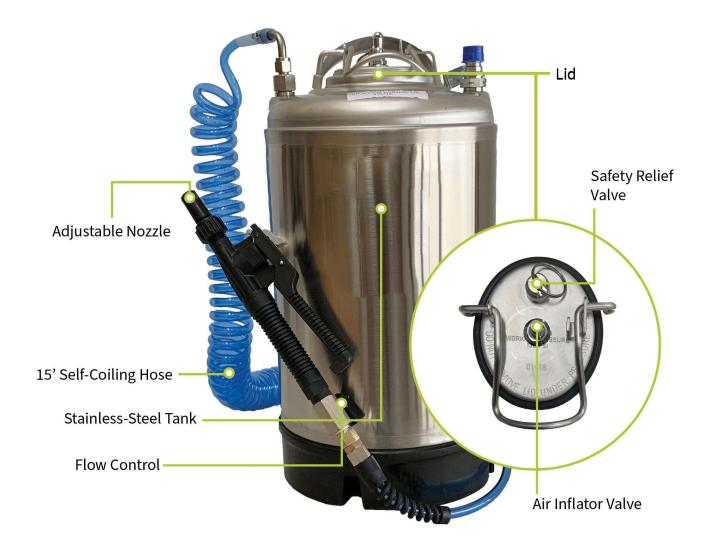
**TO OPEN**: Pull the safety relief valve ring to release air pressure. Lift the lever and push down firmly. The lid will drop down slightly and become loose. Turn the lid either direction a ¼ turn and tilt to pull the lid out of the opening.
